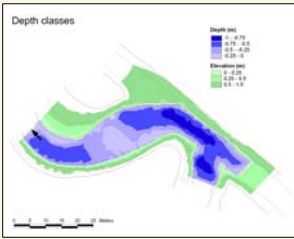
4 depth classes obtained from subtraction of riverbed DTM and low water level (~0,66 m 3 /s)
